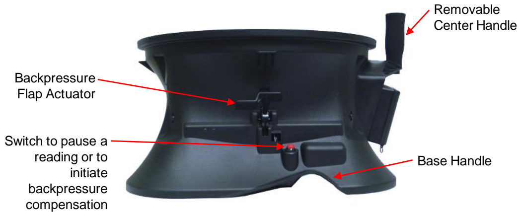
Figure 3: Features of the Model 8380 Base, Side View
