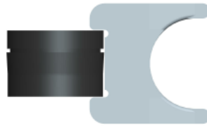
Figure 4-10: Replace Mesh in Filter Holder
